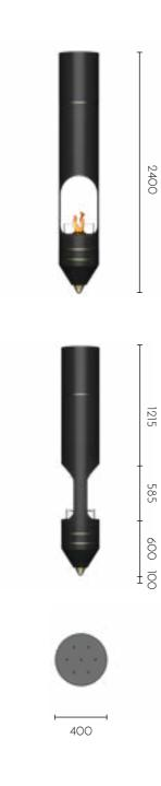
**Dimensions** 400  $\varnothing$  x 2400 h mm | 15.7  $\varnothing$  x 94.5" h Weight 110 kg | 242 lbs
