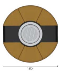
**Dimensions** 1510 Ø x 400 h mm | 59.4 Ø x 15.7" h Combustion zone 654 Ø mm | 25.7 Ø"
