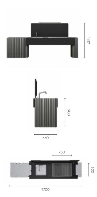
**Dimensions** 2700 w x 660 d x 1457 h mm 106.3 w x 26 d x 57.4" h Weight
