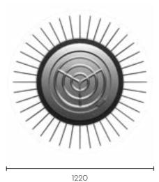
Dimensions 1220  $\varnothing$  x 345 h mm | 48  $\varnothing$  x 13.6" h Combustion zone 654  $\varnothing$  mm | 25.7  $\varnothing$ "
