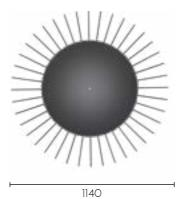
Dimensions 1140 ∅ x 330 h mm | 44.9 ∅ x 13.9" h Combustion zone 702 ∅ mm | 27.6 ∅"
