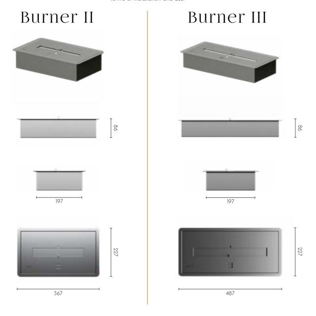
Dimensions Burner II 367 w x 227 d x 86 h mm | 14.4 w x 8.9 d x 3.4" h
